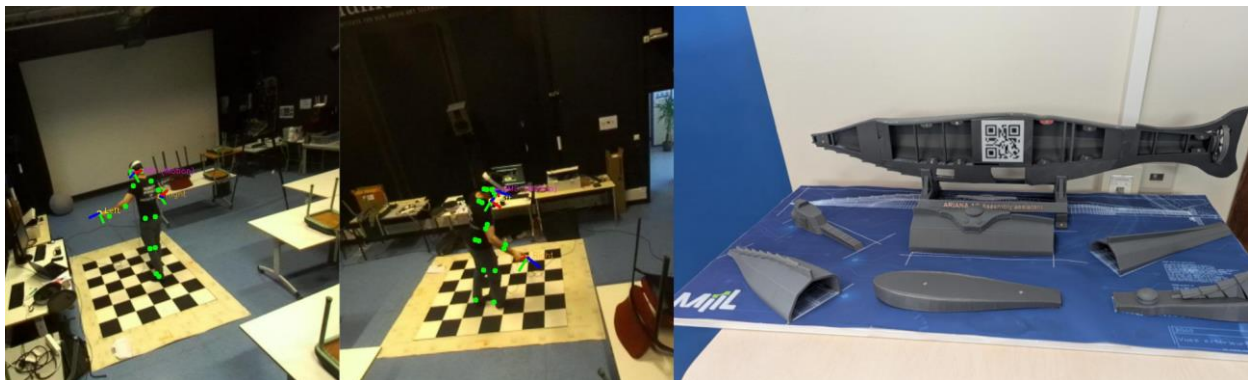
Figure 1 — Existing modules available for the project. Left: ISIA Lab calibration and synchronized multi-video acquisition system. Right: MiiL AR/MR assembly guidance prototype using a physical scale model.
